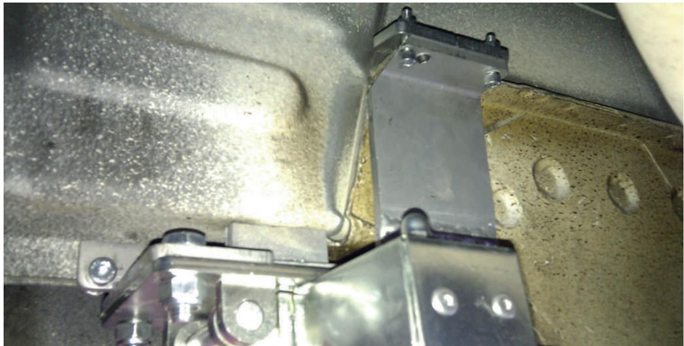
Put the adapter as far forward as possible. If necessary, remove any sealing material for greater adherence. Use a bottle jack to fix the bracket in the correct position and make an 8 mm side hole, then fix with a bolt.
